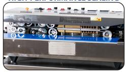
Powerful heater with precise temperature control (0–300°C) enables fast, reliable sealing across diverse film types & ideal for strong, consistent bonds.
