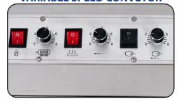
Adjustable sealing speeds up to 12m/min, maximizing throughput while maintaining seal quality.
